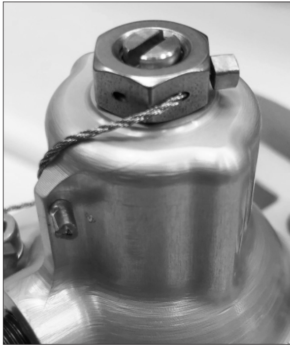
Figure 9-2 - Jam Nut Safetying
