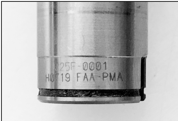
Figure 2A - Rotor Inspection Marking
