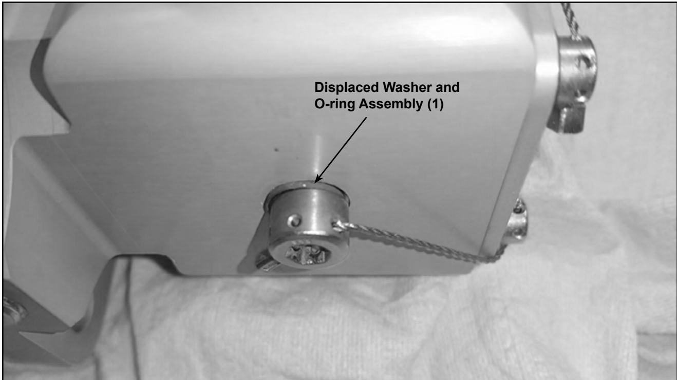
Figure 2 - Displaced Washer and O-ring Assembly
