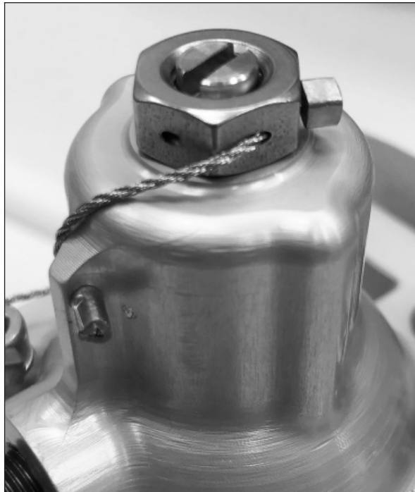
Figure 9-2 - Jam Nut Safetying
