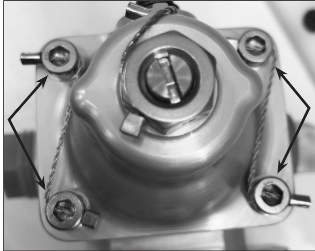
Figure 9-3 - Cap Screw Safetying
